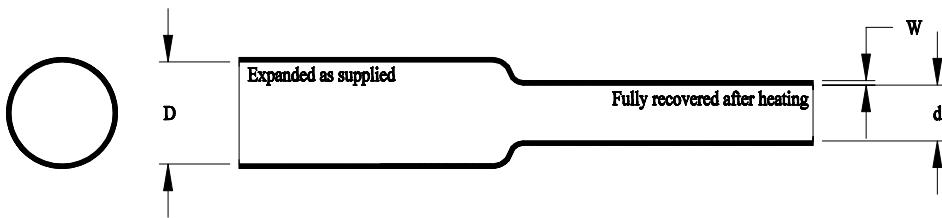
This specification covers the requirements for one type of single wall, electrical insulating, extruded tubing whose diameter will reduce to a predetermined size upon application of heat in excess of 110°C (230°F).
