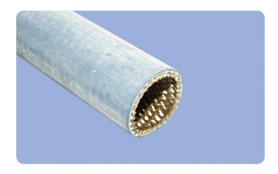
**Ben-Har™ 1151-FRB** is a rugged, flame-retardant, silicone rubber coated sleeving that provides excellent cut-through and abrasion protection for wiring systems in applications with temperatures ranging from -70°C to 200°C. Because the specially formulated silicone rubber is extrusion coated over the non-combustible fiberglass braid, it results in a reinforced sleeving that is superior to ordinary dip-coated sleeving and unreinforced rubber or plastic tubing.
